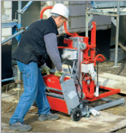
Transport – Due to rubber tyre wheels the base unit can be transported easily on the jobsite.
